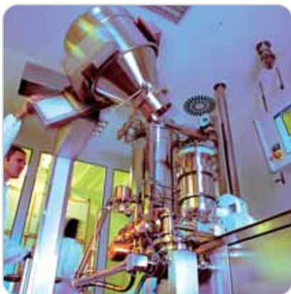
Pharmaceutical milling at Siemens Axiva GmbH & Co. KG, Frankfurt, Germany
